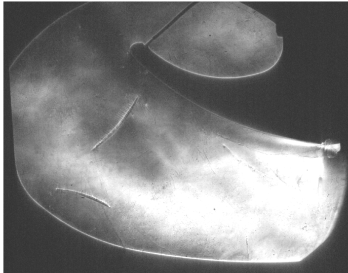
Fig. 8: Flow visualization for the case with the medium flow through the seal
