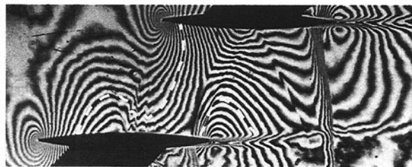
Fig. 3: A compressible flow at M_1 = 0.92, \alpha = 1.2 - experiment of IT AS CR, source: [3]
