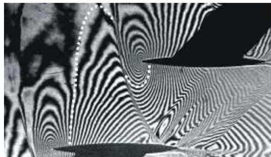
Fig 9: Experimental data, M_{\infty} = 0.982 , \alpha = 0^\circ
