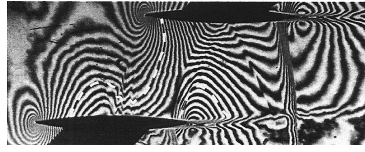
Fig. 13: Compressible flow in the DCA 8% cascade, experiment IT CAS CR, Mach number isolines, M_1=0.863, \alpha=0^\circ , author: R. Dvořák [1]
